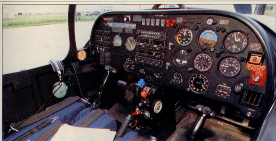
Students sit on the right, so the throttle and flaps can be operated with the left hand.
